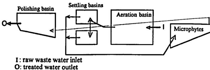
Fig. 1 : Diagram of the treatment plant.
